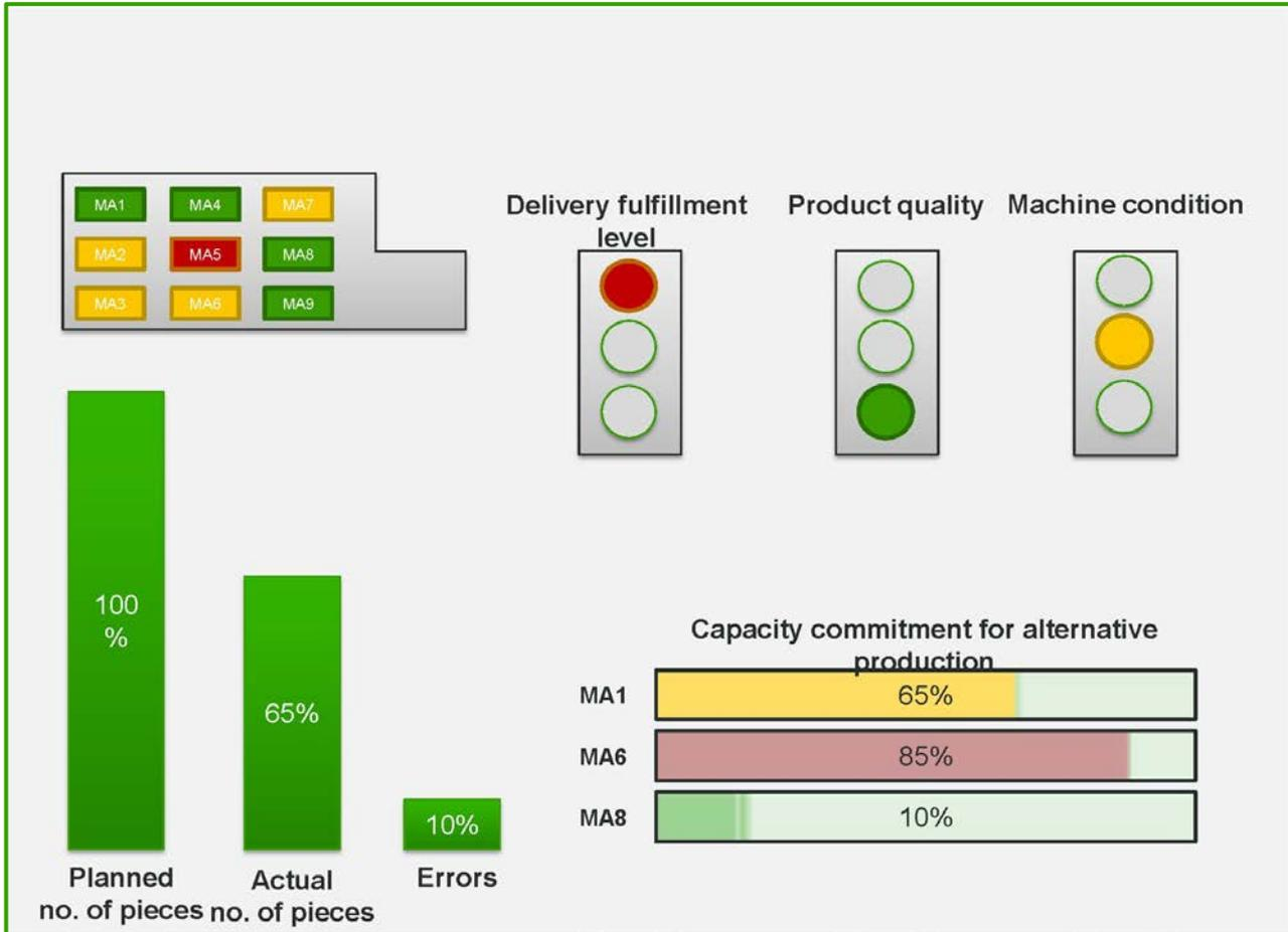
Figure 3: Dashboard for machine monitoring (schematic diagram)
