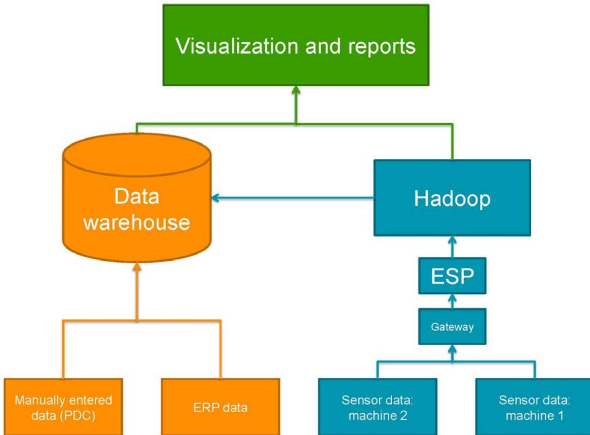
**Figure 2:** Architecture for the analysis of industrial sensor data
